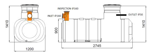
Manhole diameter: **600mm**, Treated wastewater pump: **Pedrollo Top2 Vortex**
